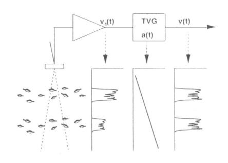
where  $v_1(t)$  = uncompensated voltage, a(t) = receiver gain, v(t) = compensated voltage
