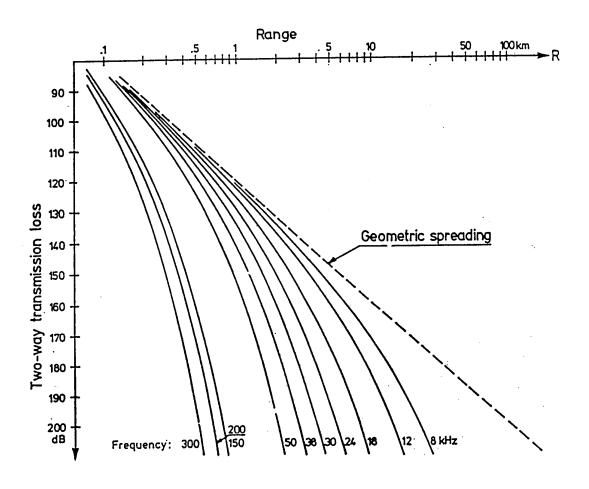
$$V_o = SL + G_1 + TS + 2D_i(\phi, \theta) - 40log(r) - 2\alpha r + \frac{G_{tvg}}{G_{tvg}} + G_{rec}$$
